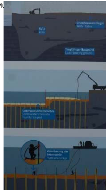
The Berlin municipal authorities plan to drive 1,200 piles into the will need to work for extended periods beneath the fast-flowing Kupfergraben canal.
