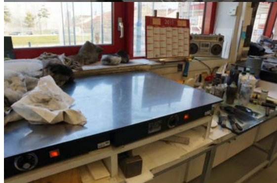
Ink preparation; the inking table features a preheating function to reduce ink viscosity
