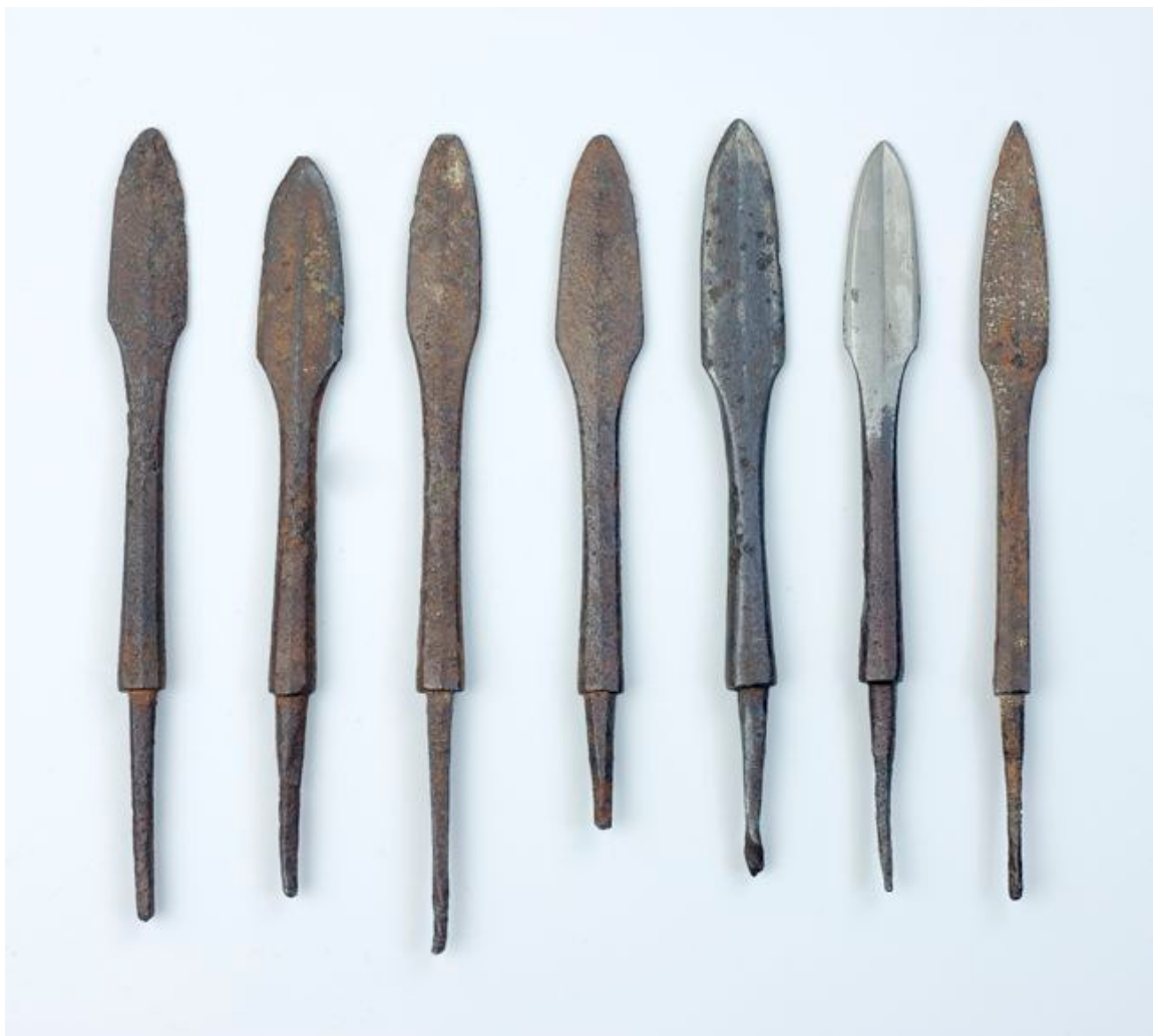
Various plum needle arrowheads from my own collection. The sixth was polished, revealing a tight forge-folded construction, just like on
