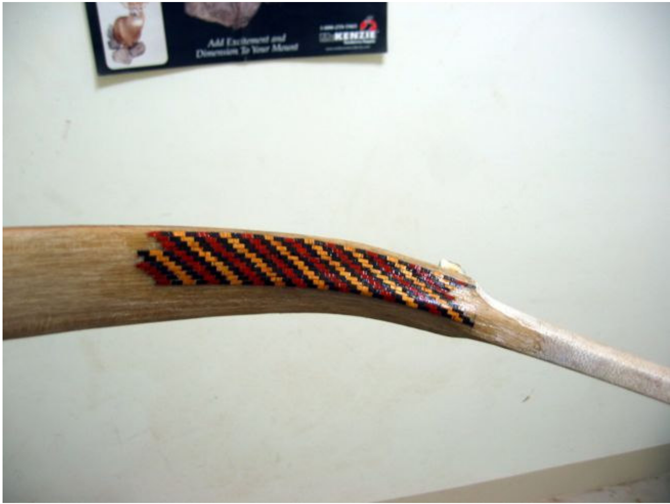
Glueing the strips to the inside of the knee.
