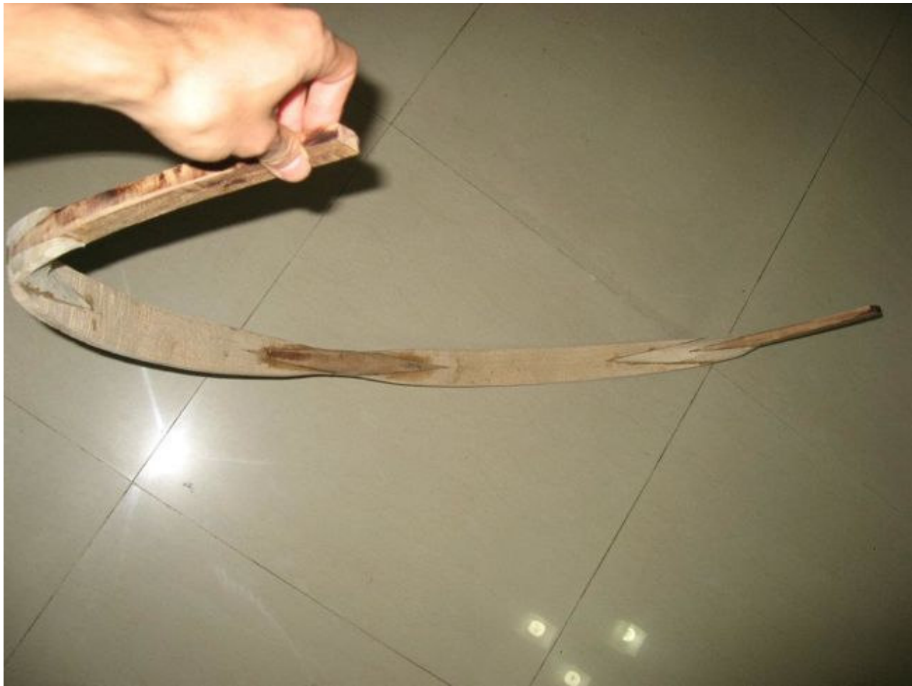
A finished core. All parts need to be in perfect alignment, which with so many splices is quite a feat.
