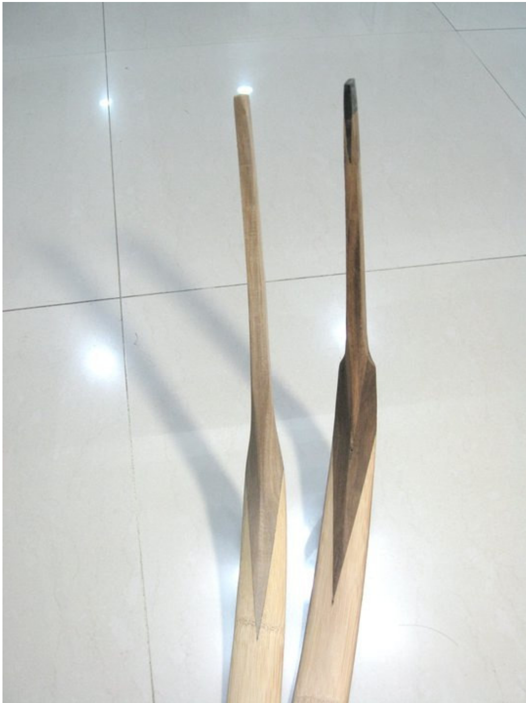
Expertly executed v-splices.
