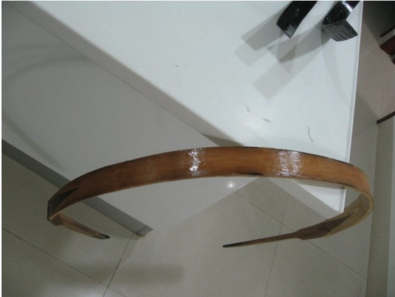
The belly of the core is covered with glue, as is the horn, before the two are joined.
