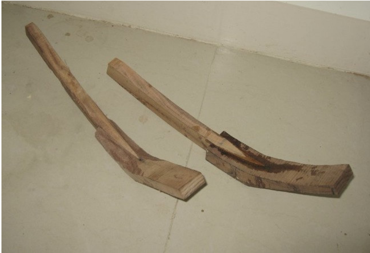
Two ears spliced into their knee pieces. These knees are referred to as 腦 in Chinese, literally the "brain" of the bow.
