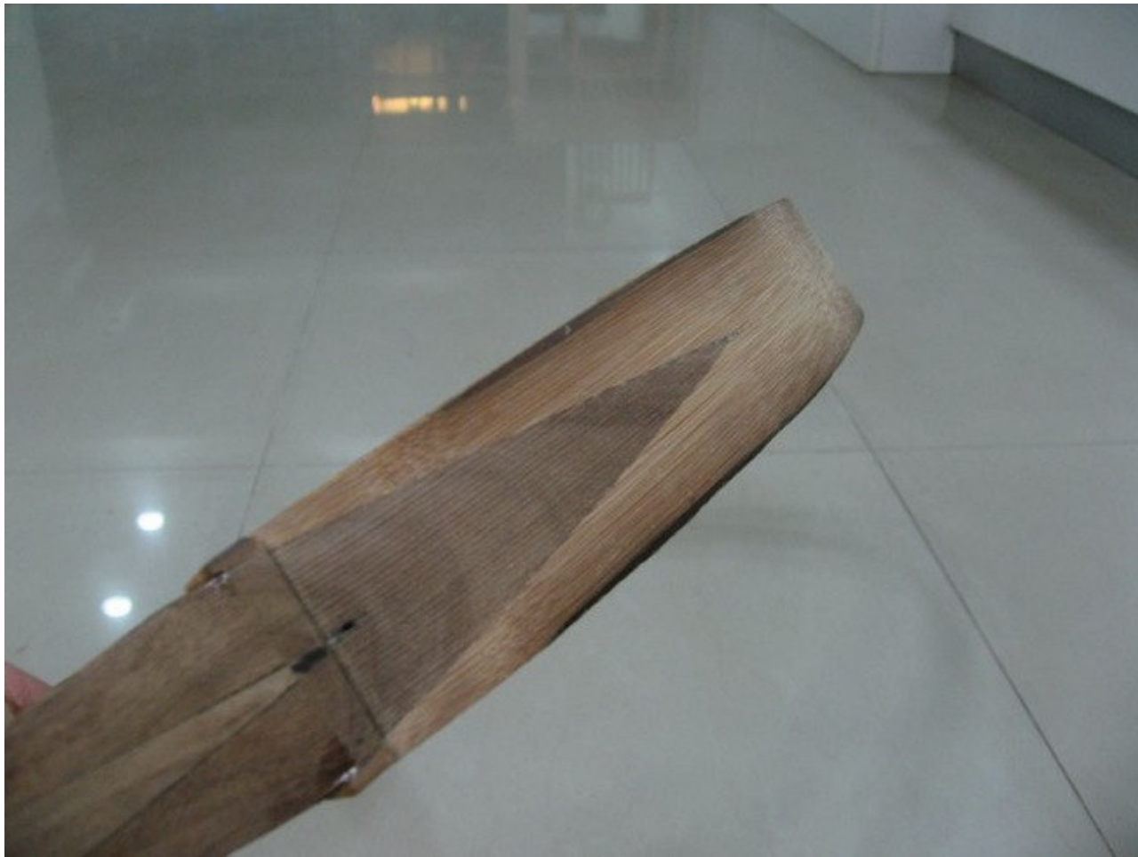
The belly side of the core is scored to increase the surface for glueing.
