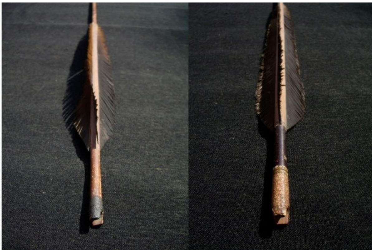
Left: the tail of a hunting broadhead arrow with twisted fletchings. Right: the straight fletchings on a target arrow's tail. Author's collection.
